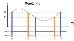
The alarm goes off when the measurement is outside the low and high thresholds.
